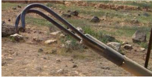
Damaged Heavy rake
