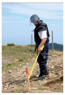
[A deminer searching for submunitions in Serbia in 2007. The detector is use is a stick detector, only capable of detecting fairly large ferrous targets.]
