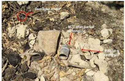
[The copper cone of the shaped charge inside the M77 was visible at one end, and the high explosive fill at the other.]
