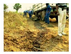
The picture shows the crater in the foreground and the damaged truck beyond. The detonation removed the wheel and damaged the wheel hub and track-rod. The front bumper, wheel-arch, cab door, steering wheel and internal fittings were damaged.
