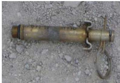
[The investigators indicated that the “percussion cap” screwed to the left end of this was the “detonator”. It is not. This fuze does not have a detonator attached.]
