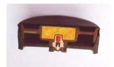
The injuries resulting from stepping on a PMA-3 vary from bruising to traumatic amputations. The picture above shows why this happens. It shows a cut-away section through a PMA-3. The 35g Tetryl is in the top and centre of the mine. The area of pressure-plate surrounding the HE is actually larger than the area of pressure-plate over it. If a victim is fortunate, they step on the pressure plate but the explosive charge is not beneath their foot.
