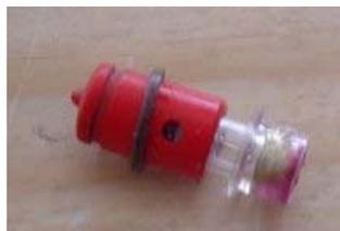
In several cases the ball bearing mechanism has jammed and although the balls are lined up with their exit holes, they have not moved sideways to allow the spring-loaded pin to drop. In these cases, they could move at any time – which may explain why the mine went off as the supervisor unscrewed the booster charge. The picture alongside shows the mechanism with the pin just visible above the detonator.
