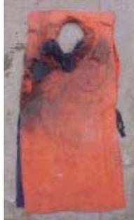
The investigators decided that there were two possible reasons for the accident. Either the victim inadvertently applied pressure to the mine while unscrewing the booster or the "oxidisation of friction sensitive crystals from the booster" made the mine detonate as he worked.
