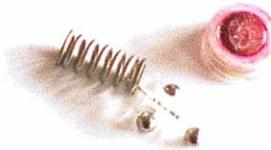
[The detonator/percussion cap is set into clear plastic as shown in the picture above, which shows the entire metal content of the mine].
